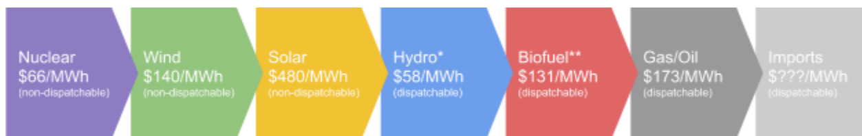
Figure 5.7-2. Dispatch order by resource type based on price and dispatch capability. *Hydroelectric generation is used in Ontario for peaking and intermediate generation with hydro pumped storage (IESO, n.d.). **Biofuel plants are also employed for peak demand generation (Murray, 2017).
